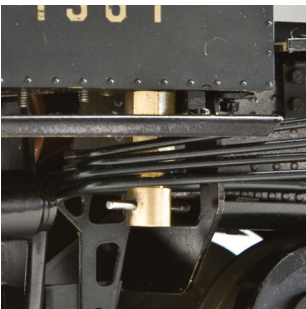
Blow Down Valve
